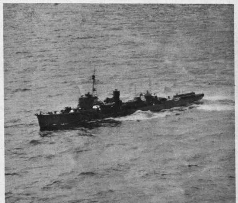
Coastal minelayer , probably of Sokuten Class, has parallel stern racks. Simple bridge, forecandle deck, mainmast make design typically Jap.
